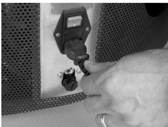
Figure 17 – Disconnect the stove from the electrical mains
