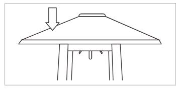
**STEP 6:** Place Reflector (1) on the Flame Screen (2) and fix the connection with 4pcs M5 CAP NUT (AA).
