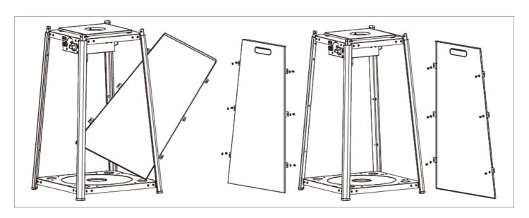
**STEP 3:** Obliquely insert and attach 2pcs Side Panels (12) and 1pc Rear Panel (10) into tank housing using 18pcs M5 self-tapping screws and washers (CC). Best affix two opposite sides first, fastening the screws diagonally.
