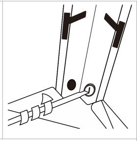
STEP 7: Place the whole upper parts to top of tank housing assembly. Make sure match the top ends of tank housing assembly with the bottom slot of Support Bar – Upper (3). Match the threaded holes and fix each connection with 2pcs M5 Screws and Washers (BB)
