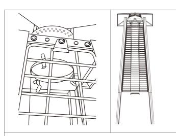
**STEP 10:** Assemble Mesh Guard (4) in the front. Loose 4pcs screws to keep 4pcs Guard Fastening Plates down and firmly in place.
