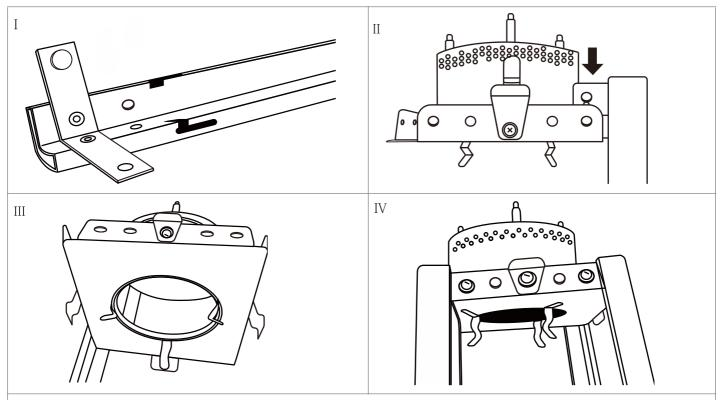
**STEP 5:** Attach Flame Screen (2) to the top of Support Bar-Upper (3) and fix the connection with 2pcs M5 screws and washers (BB), (See Figurel, II).
