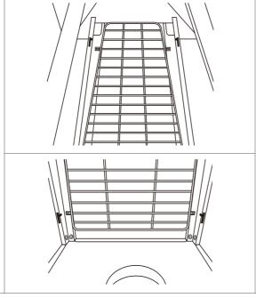
**STEP 8:** Insert 6 projecting ends of each Mesh Guard (4) into the seat slots of Support Bar–Upper (3) as shown in picture. Fix all Mesh Guards (4) except the front side.
