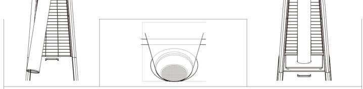
**STEP 9:** Fix Rubber Ring (6) into the bottom of Glass Tube (5). Insert the top end of glass tube into the bottom hole of Flame Screen (2) as much as possible. Keep glass tube vertically and sit it in the hole of Plate Cover (8). **NOTE: GLASS TUBE IS FRAGILE PART, PLEASE HANDLE GLASS TUBE CAREFULLY AND SLOWLY!**
