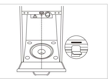
**STEP 11:** Insert the feet of door into the bottom slots. Attach the Chain (7) to the hook of Burner Assembly (9) and close the door.
